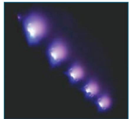
Figure 29a. Cylindrical small ion sources of EH-200 type [67a] placed as a linear array to substitute one long linear end-Hall source. All five ion sources utilize one Hollow Cathode for neutralization of ions.
